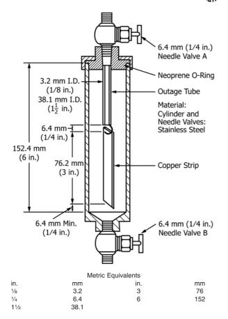
FIG. 1 Copper Strip Corrosion Test Cylinder
