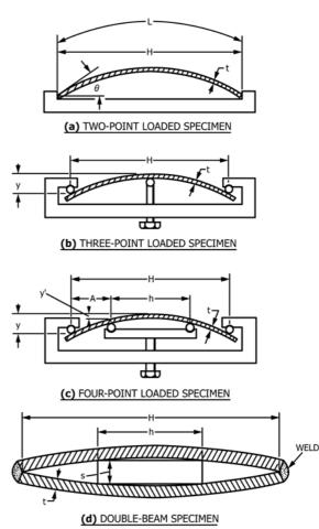
FIG. 1 Schematic Specimen and Holder Configurations
