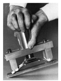
FIG. 2 Stressing Jig and Two-Point Loaded Specimen with Holder (approximately 1/4 actual size)
