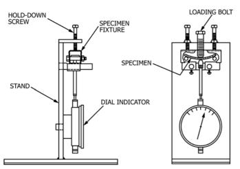
FIG. 3 Specimen Loading Apparatus for Three-Point Loaded Beam Specimens with Integral Deflection Gage
