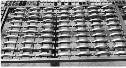
FIG. 4 Bent-Beam Specimens on Atmospheric Exposure Rack
