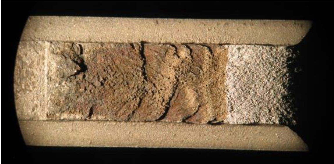
Figure 12: Example of Invalid Test due to Edge Cracks Using Low-Angle Fiber Optics Illumination (See Paragraph 11.6.1[e])
