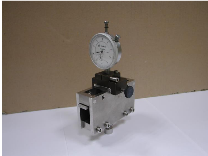
Figure 3: Loading Jig with Dial Gauge Attached for Measurement of Deflection
