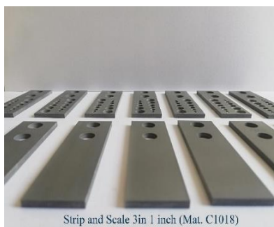
Strip and Scale 3in 1 inch (Mat. C1018)
