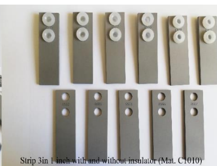
Strip 3in 1 inch with and without insulator (Mat. C1010)
